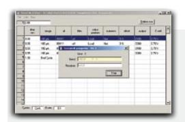
Editor for time files, and transmitting to DECADE II: Time file editor is a tool for writing and transmitting time files to the detector.
