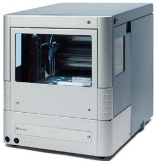
The AS 110 is a new generation autosampler. It is a fast, robust and easy to use autosampler without compromising accuracy and reproducibility. The AS 110 includes indispensable features for the highest injection performance. It has a dual needle with positive headspace pressure, extensive wash routines for minimal carry over and 3 injection modes including  $\mu$ L pick-up mode for zero sample loss.
