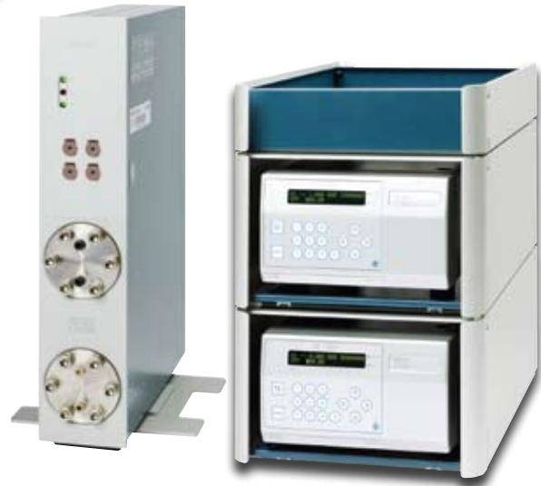
The compact Organizer OR 110 includes an extremely efficient degasser and pulse damper. It can be upgraded with a second pulse damper. The power supply for all ALEXYS™ components comes from the OR 110 avoiding grounding loops.
