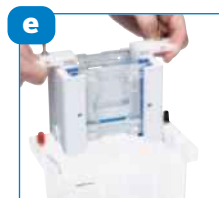
Transfer to tank and fill with buffer
