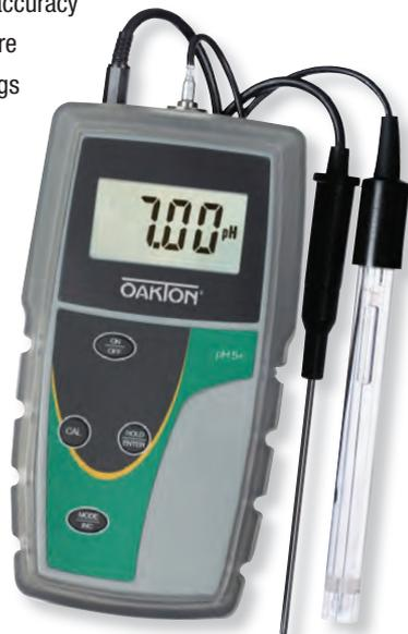
**Meter includes:** ATC probe, protective rubber boot, and batteries.
