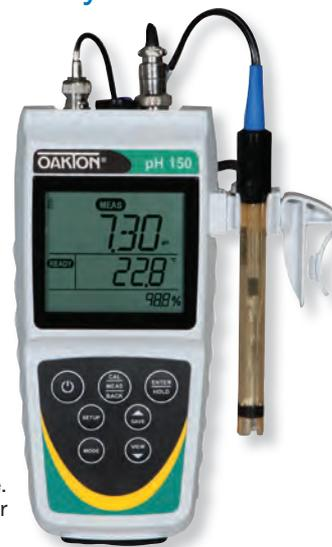
View more simultaneously with large, three-line LCD providing pH or mV measurement with temperature and calibration % slope. Get faster calibration with auto buffer recognition which identifies the correct pH buffer. Be more accurate with up to six calibration points from USA, NIST, and DIN pH buffer sets and automatic temperature compensation (ATC).
