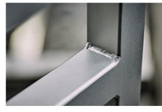
Ill. left assembly production of stainless steel components (TIG welding) Ill. top hygiene requirements – edges to prevent dirt accumulation Ill. middle primate-safe cage closures Ill. bottom clean and corrosion re-
