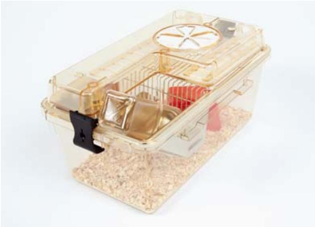
Complete IVC 2 L type cage incl. cage, stainless steel lid, filter level, filter top incl. CO<sup>2</sup> membrane and water bottle
