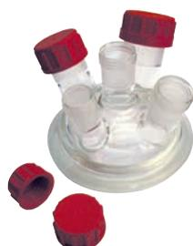
Precision ground lid and vessel flanges combine with PTFE collar and FEP-encapsulated O-ring to offer superior sealing performance.
