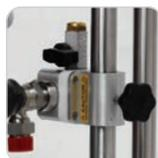
Quick-release PEEK coupling allows rapid exchange of vessels without the use of tools. Operates over the temperature range -30 °C to +180 °C (jacket temperature).
