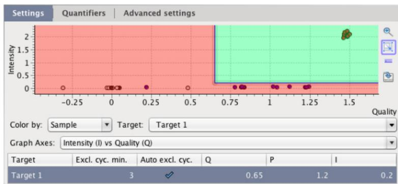
The dots represent individual amplification curves in your experiment. All dots that are within the top right of the graph are called positive and will be subject to normalization determined in **Advanced Settings**.
