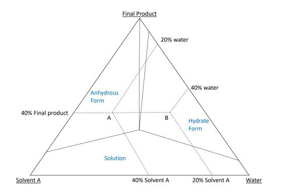
Figure 14. Schematic of a typical final product-hydrate phase diagram
