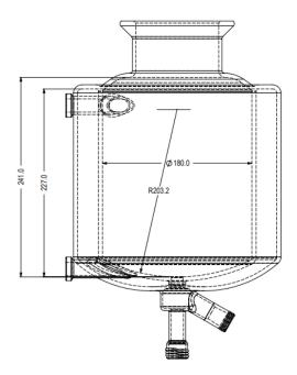
Figure 12. Radleys Process Vessel (torispherical geometry)
