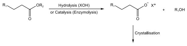
Figure 9. Reactive crystallisation: base catalysed hydrolysis of an ester to form a carboxylate anion and subsequent crystallisation
