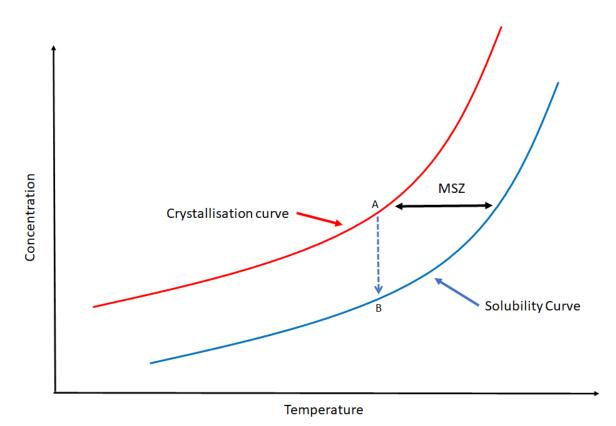
Figure 1. Diagram showing the Meta Stable Zone which exists between the solubility and crystallisation curves, and is dependent on the temperature and concentration of the process
