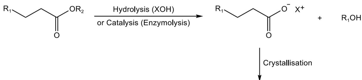
Figure 9. Reactive crystallisation: base catalysed hydrolysis of an ester to form a carboxylate anion and subsequent crystallisation
