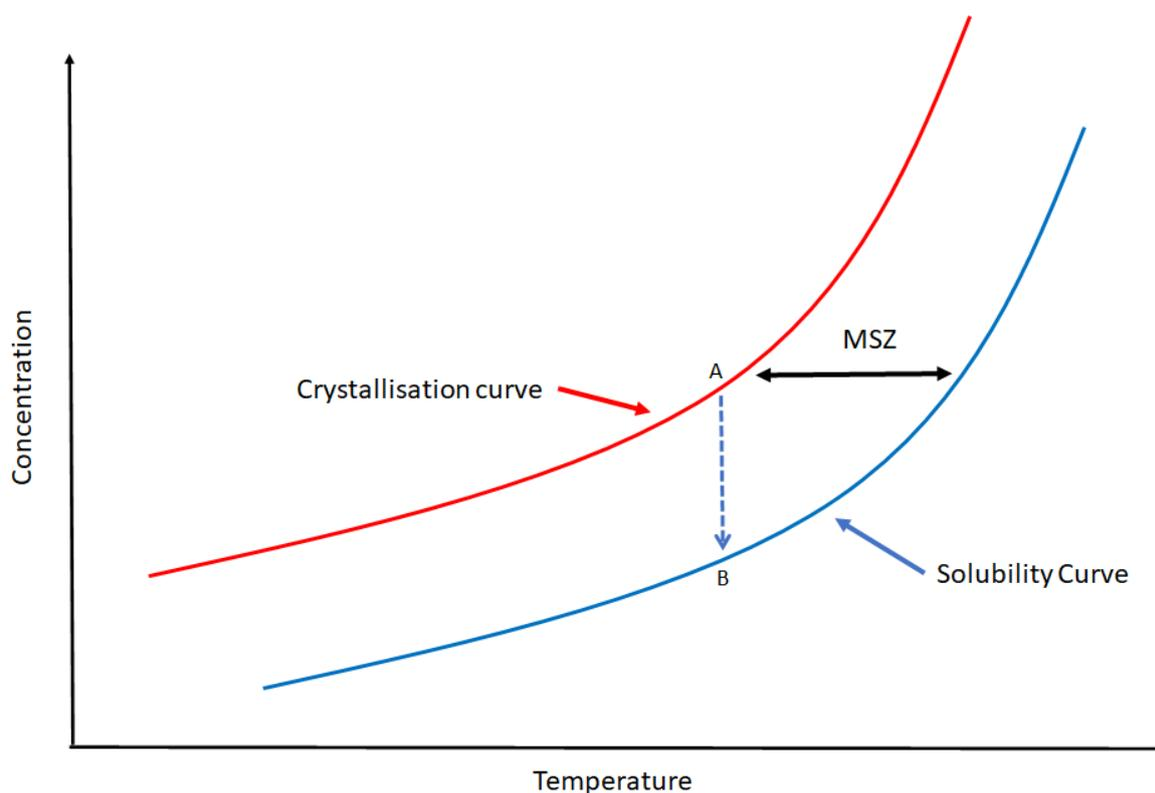
Figure 1. Diagram showing the Meta Stable Zone which exists between the solubility and crystallisation curves, and is dependent on the temperature and concentration of the process
