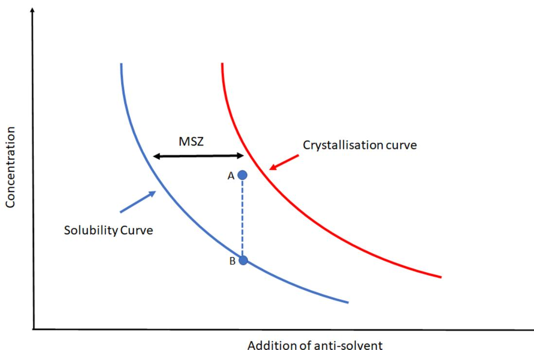
Figure 3. Normal anti-solvent addition scheme
