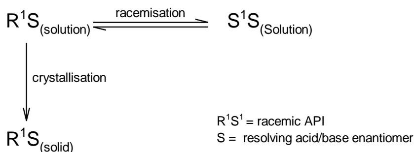
Figure 10. Typical diastereomeric salt resolution
