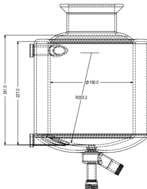
Figure 12. Radleys Process Vessel (torispherical geometry)
