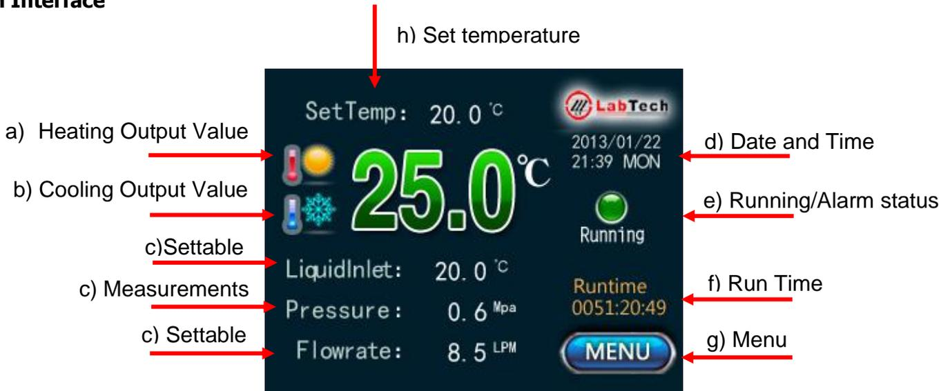
a) Heating output indicator: the icon is switched ON when the unit is heating.
