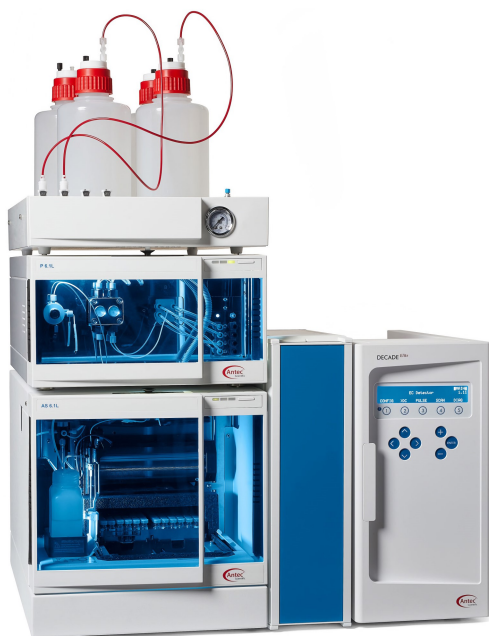
Figure 5: Recommended instrument configuration for this application: the ALEXYS Carbohydrate Analyzer with Solvent Switch Valve. The system consists of a P6.1L pump with integrated degasser and Solvent Switch Valve (SSV) for the option to run step gradients or automated column clean-up, an AS6.1L autosampler, an ET 210 Eluent tray for helium blanketing, and the DECADE Elite electrochemical detector. A CT 2.1 column oven with broad temperature range can be added optionally for separations under near-ambient temperatures. The ALEXYS Carbohydrate Analyzer can be operated under different Chromatography Data System (CDS) software: DataApex™ Clarity™ CDS (version 8.3 and up) or Thermo Scientific™ Chromeleon™ CDS (version 7.2 SR 5 and up).
