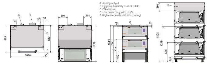
Note: The dimensions above only apply to the 230 V version. The heights of the bases of the 115 V version are slightly different (high base = 406 mm instead of 450 mm; low base = 140 mm instead of 130 mm).
